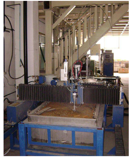
Figure 4 Water jet cutting equipment
