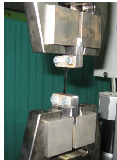
Figure 5 Fastening of the specimens into the test machine jaws
